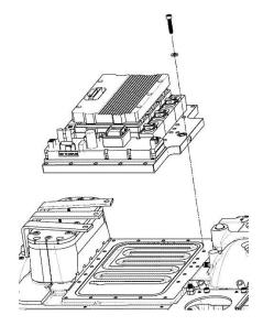
This kit contains the Inverter, O-rings, and fasteners. Please refer to our Service Manual for details regarding the replacement of the Inverter.
