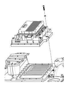
This kit contains the Inverter, O-rings, and fasteners. Please refer to our Service Manual for details regarding the replacement of the Inverter.
