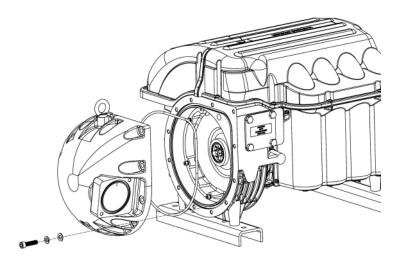
This kit contains the Second Stage Housing as well as the required O-rings and fasteners. Please refer to our Service Manual for details regarding the replacement of the housing.
