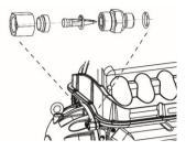
This kit contains the Strainer and O-ring for the Cooling Adapter. Please refer to our Service Manual for details regarding the replacement of the Interstage Pipe O-rings and fasteners.
