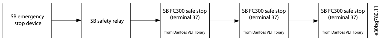
Illustration 9: Safety-related Block Diagram
