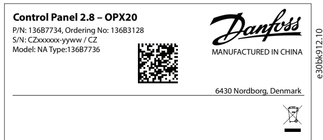
Illustration 54: Example of a Control Panel Label
