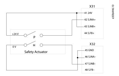
Illustration 8: STO Connection Example for Using Different Polarities
