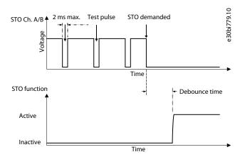
Illustration 1: Test Pulse Filtering
