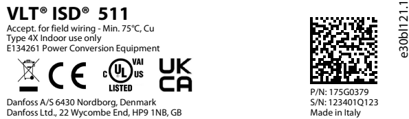
Illustration 65: Tracing and Conformity Label on the Electronic Cover of ISD 511
