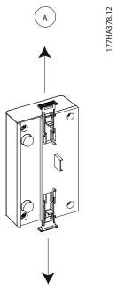
Illustration 3.2 Removing the EtherNet/IP Option
