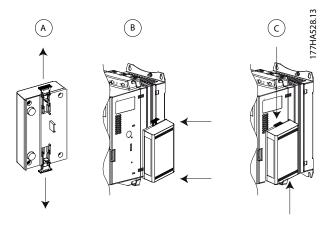
Illustration 3.1 Installing the EtherNet/IP Option
