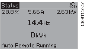
Figure 5.2: Step 1: Turn on the adjustable frequency drive (On LED lights)
