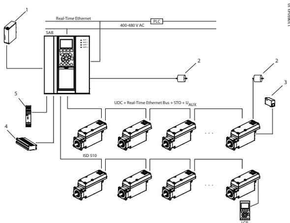
**Illustration 2.7 Overview of the ISD 510 Servo System and Components**
