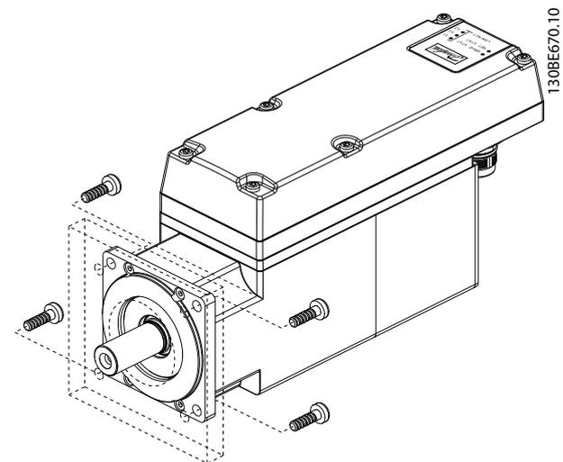
Illustration 6.20 Mounting of Size 1, 1.9 Nm, Size 2, 2.9 Nm, and Size 2, 3.8 Nm Servo Drives
