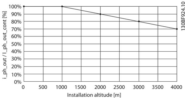
Illustration 6.19 Derating of Phase Output Current versus Installation Altitude
