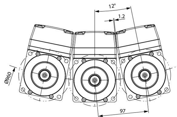
Illustration 4.1 Example of Servo Drive Installation on the Same Flange
