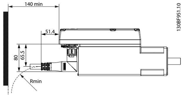
Illustration 6.36 Required Installation Distance and Minimum Bending Radius for M23 Angled Connector
