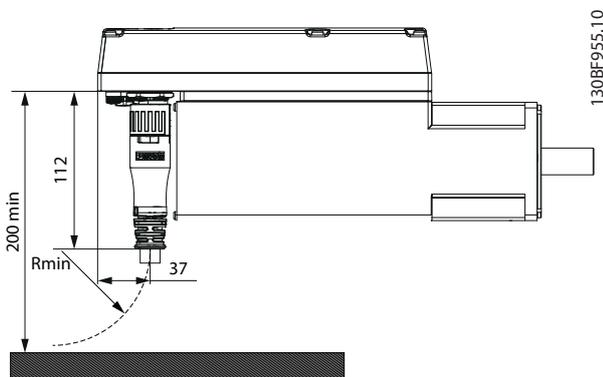
Illustration 6.35 Required Installation Distance and Minimum Bending Radius for M23 Straight Connector
