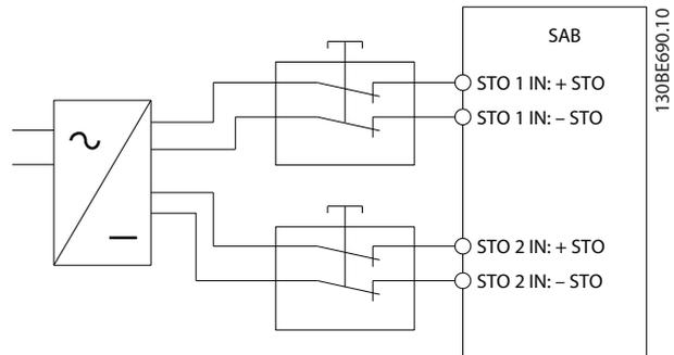
Illustration 2.10 Safety Relay with Plus and Minus Switching Output
