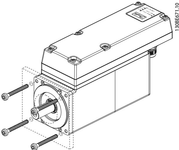
Illustration 6.21 Mounting of Size 2, 2.1 Nm Servo Drive
