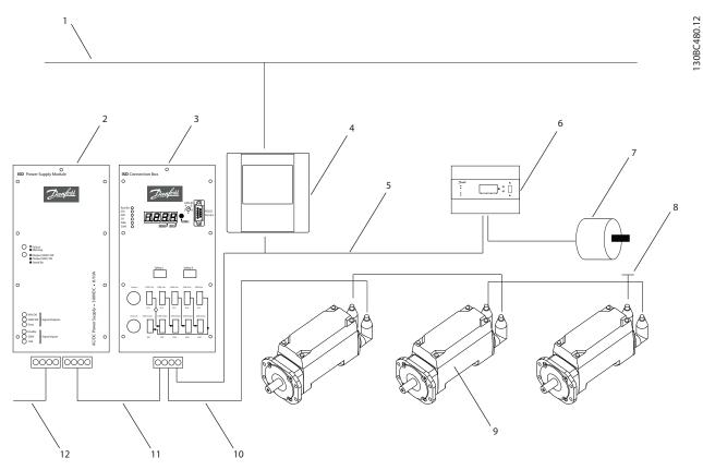
Illustration 2.1 ISD Servo System with 3 Servomotors
