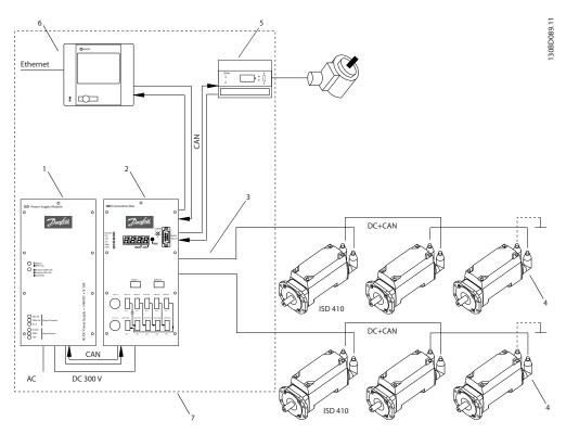
Illustration 4.2 ISD Servo System with 1 ISD Connection Box
