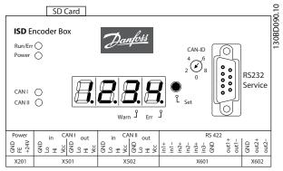
Illustration 4.4 Connections on the ISD Encoder Box
