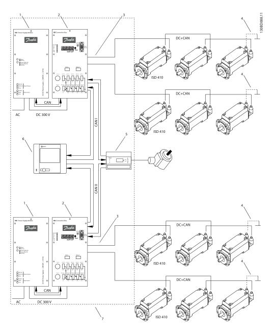
Illustration 4.3 ISD Servo System with 2 ISD Connection Boxes
