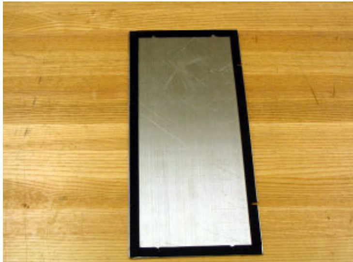
Photo 16. Top duct closing plate with gasket.
