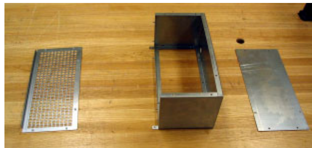
Photo 7. The top duct work partially assembled with bottom flange.
