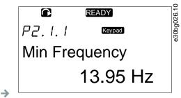
2. To go to the Edit mode, push the Menu button Right. The parameter value starts to blink.
