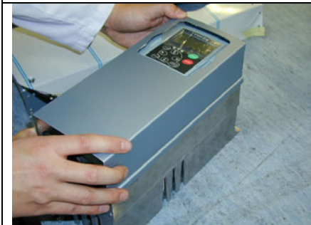
14. Fit the IP54 cover in its place; keypad end first, then cable end.
