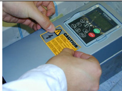
17. Attach the warning sticker (#6/#7) on the IP54 cover.
