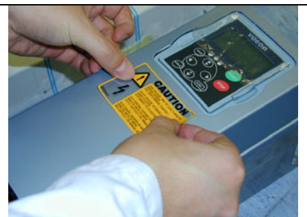
18. Attach the warning sticker (#6/ #7) on the IP54 cover.
