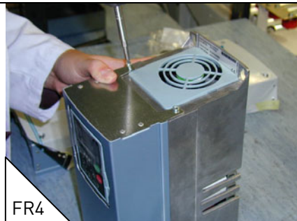
FR4 15. Use the attached screws (#5) to fix the IP54 cover on the upper end of the converter.
