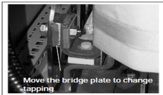
Figure 5-6. Input chokes tapping in FR13/14 units
