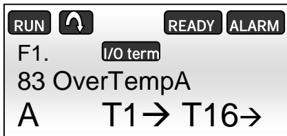
Figure 5.1-2, High temperature alarm on the NXP panel
