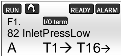
Figure 5.1-4, Low pressure alarm on the NXP panel
