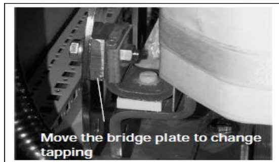
Figure 5-6. Input chokes tapping in FR13/14 units
