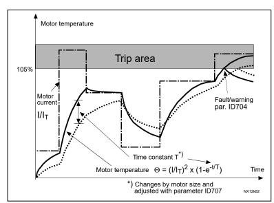
Figure 8-14. Motor temperature calculation
