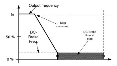
Figure 8-12. DC-braking time when Stop mode = Ramp
