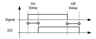
Figure 8-10. Digital outputs 1 and 2, on- and off-delays
