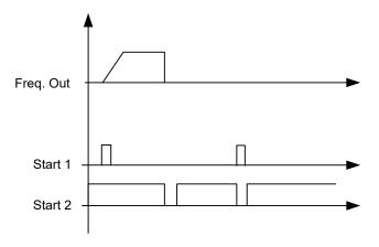
Figure 8-7. Start pulse/ Stop pulse.
