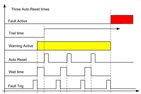
Figure 8-15. Example of Automatic restarts with three restarts
