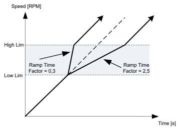
Figure 8-1. Ramp rate scaling between prohibit speeds
