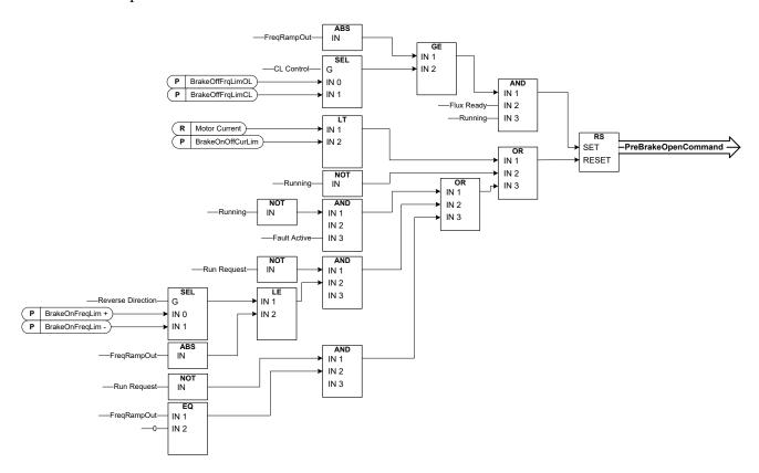
The final brake open command: It is possible that in a Master/Follower system the master drive opens the brake. Also an overriding system may do this without any control from the drive using AucControlWord1.B7. During identification run the brake will not open.
