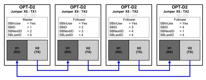
Figure 8-13. System bus physical connections with the OPT-D2 board
