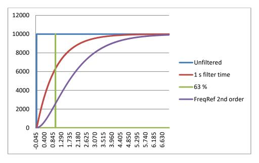
Figure 8-9. Al1 signal filtering
