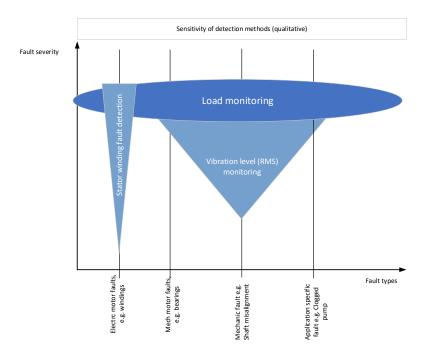
To begin condition-based monitoring a baseline must be generated. During this activity, the system captures motor stator winding speed points for each baseline. The user can define the duration, minimum and maximum speed for baseline generation. During baseline generation, 10 speed points are captured. The first and last speed point is captured based on the defined minimum and maximum speed respectively.
