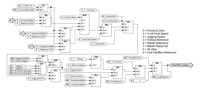
Speed reference chain before ramp control
