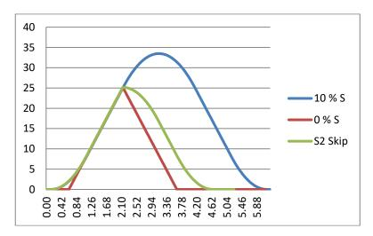
Figure 8-4. Second S curve is bypassed when reference changes at 25 Hz
