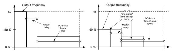
Figure 8-11. DC-braking time when Stop mode = Coasting, from nominal speed and 50 % of nominal speed.
