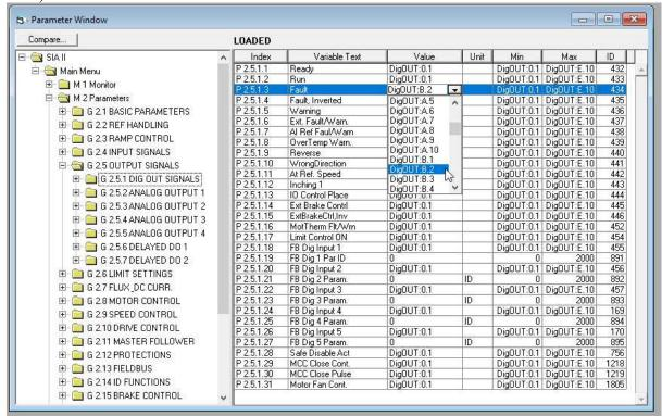
Figure 5-1. Screenshot of NCDrive programming tool; Entering the address code
