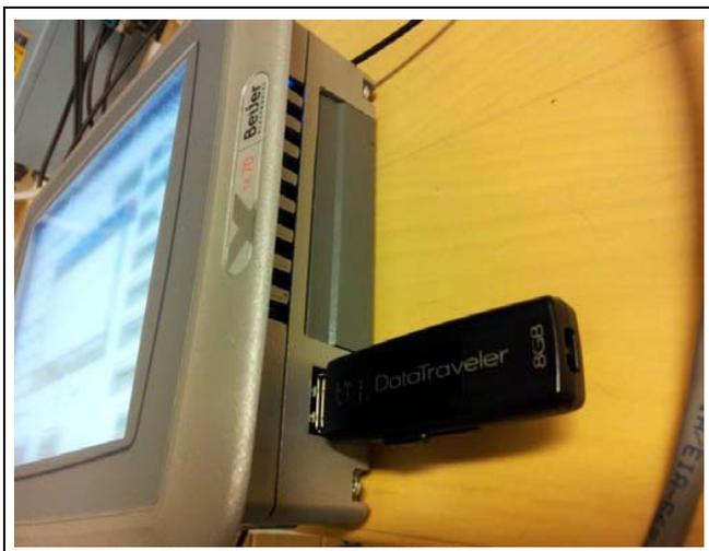
Pressing Save parameters to USB button will open a pop-up menu for choosing the name of the parameter file to be saved on the USB memory stick. The parameters are saved as an .ini file.
