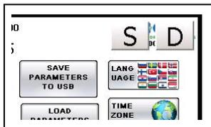
D button gives you access to the Panel diagnostic tool where e.g. CPU Load, Used Memory, Temperature and Screen info can be seen.
