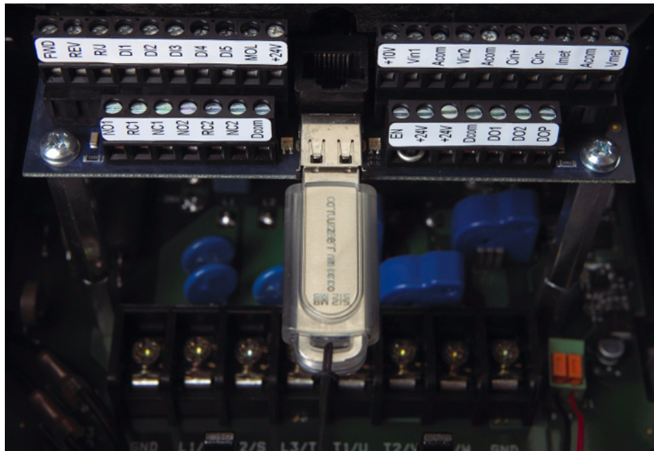
Figure 4-3: X5 Control Terminals
