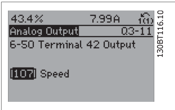
Illustration 6.1: Step 7: Use the up/down navigation keys to select between the different choices. Press [OK].
