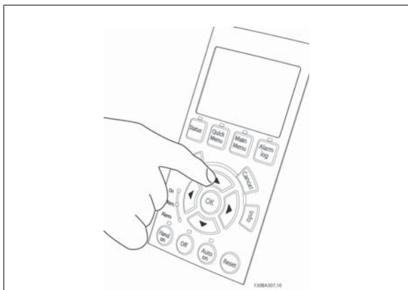
Illustration 4.46: Step 6: The speed of the motor can be seen in the LCP. It can be adjusted by pushing the up ▲ and down ▼ arrow buttons.
