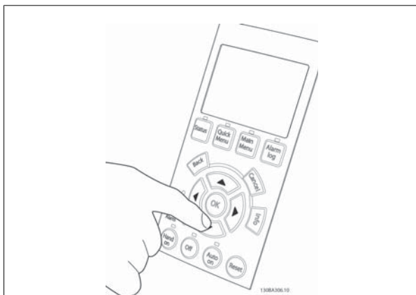
Illustration 4.47: Step 7: To move the cursor, use the left ◀ and right ▶ arrow buttons. This enables changing the speed in larger increments.
