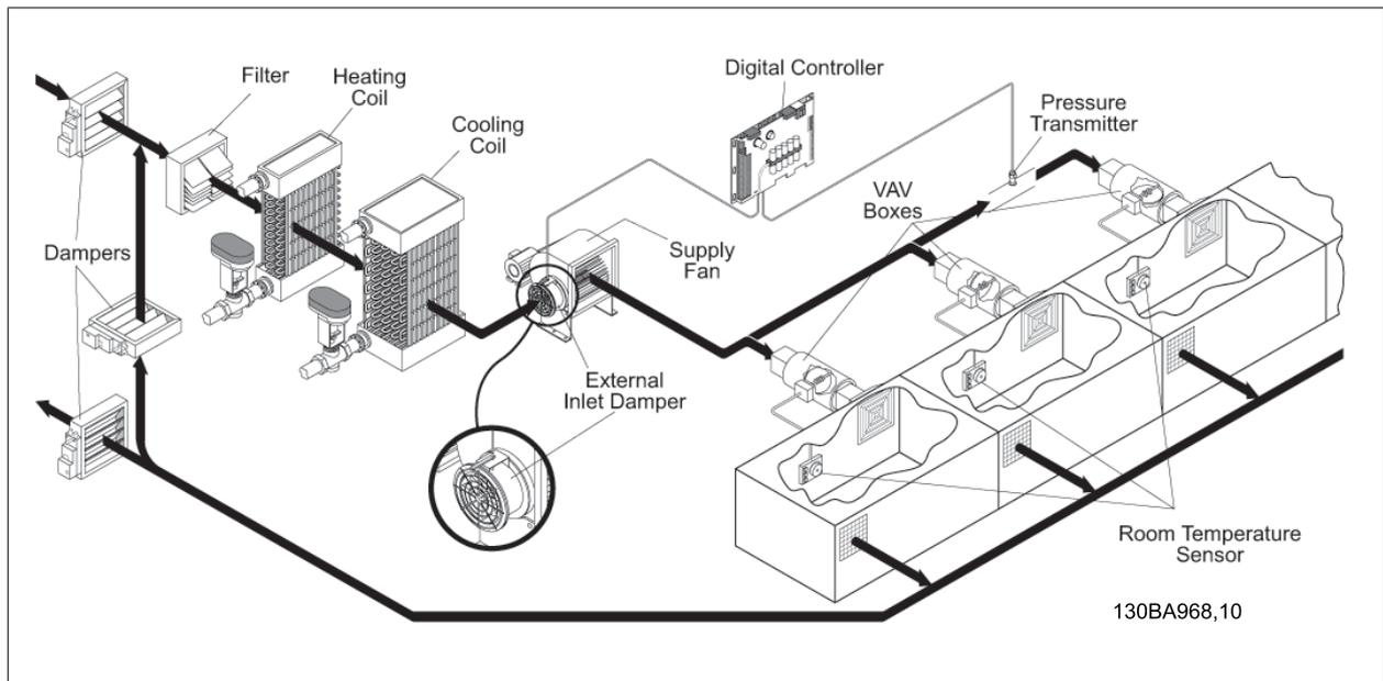
Illustration 2.1: VAV System with Inlet Guide Vanes
