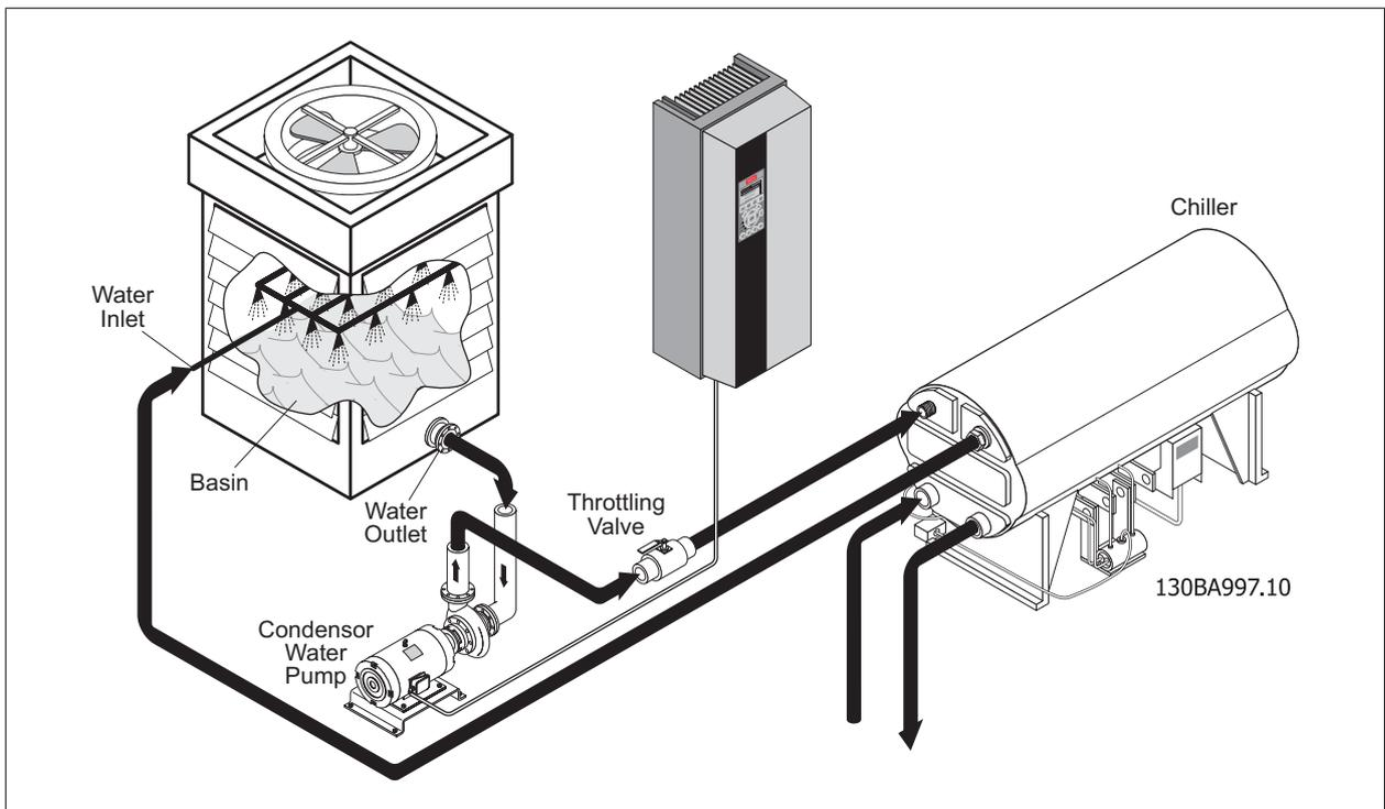
Illustration 5.5: Condenser Pump Control with Frequency Control
