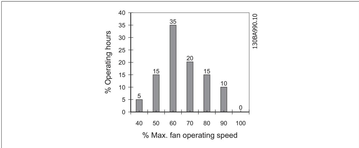
Illustration 4.3: Cooling tower operating hours and fan speed
