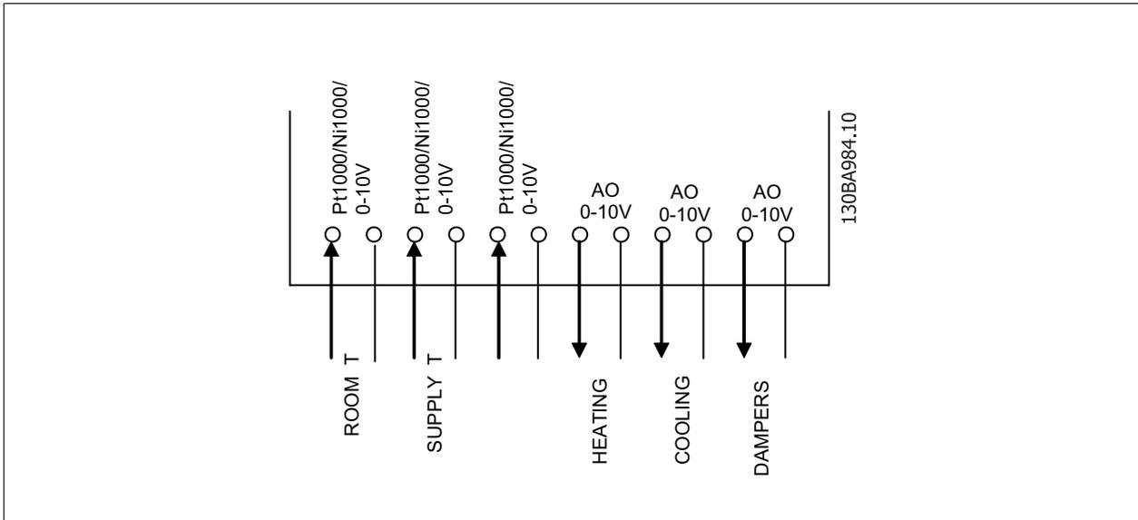
Illustration 3.5: Typical MCB 109 I/O Wiring
