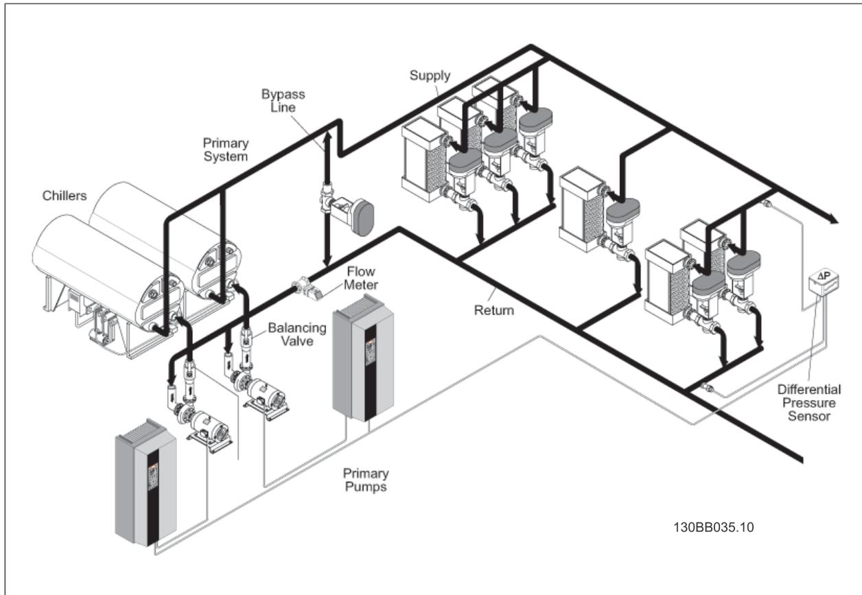
Illustration 8.2: Variable Primary Flow System with frequency converters
