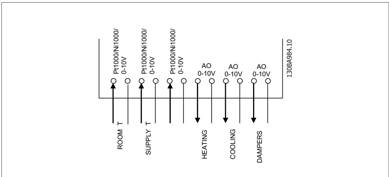
Illustration 2.10: Analog I/O Option Card Wiring
