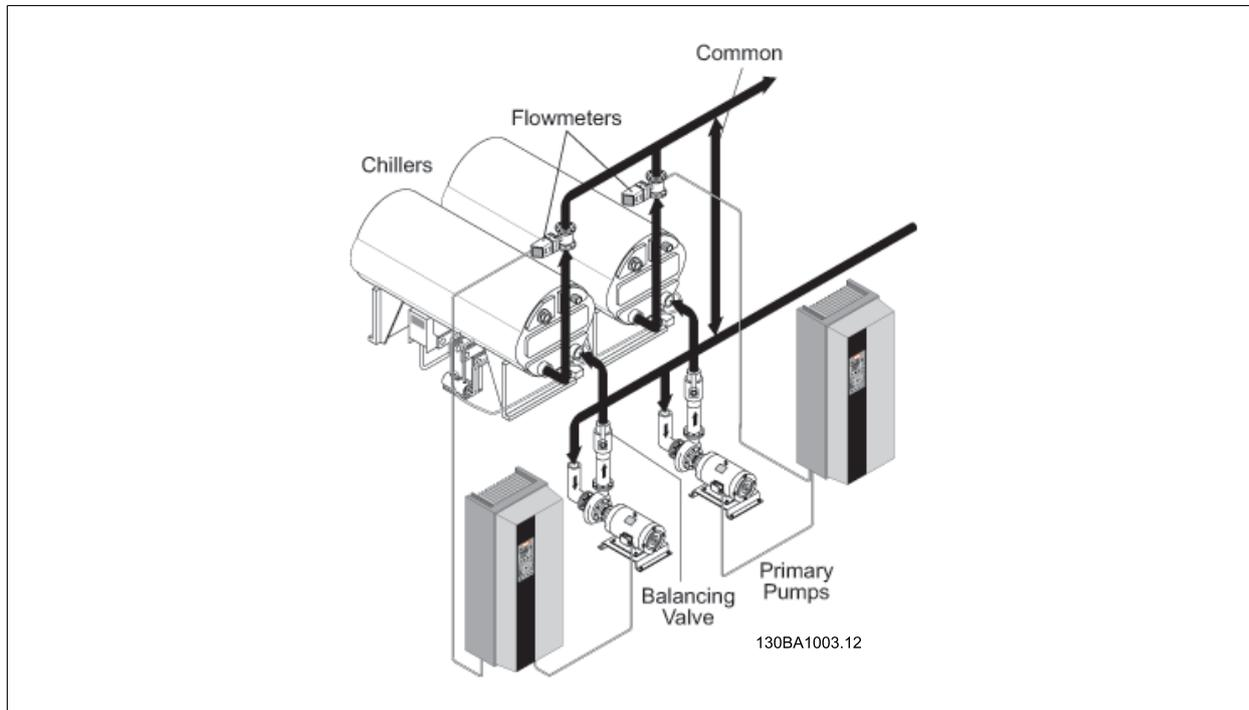
Illustration 6.5: Frequency Converters for Primary Loop Control
