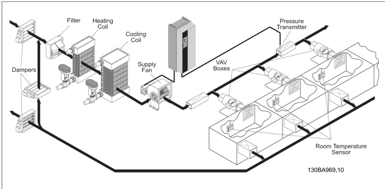
Illustration 2.2: VAV System with Adjustable Speed Drive
