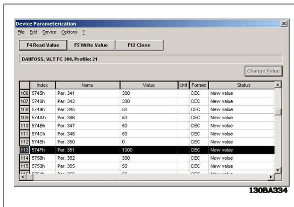
To activate the new settings with PCD, the CMD needs to read the configuration from the VLT frequency converter again. Click on the controller board and select Process data. The Process data should now be 64 bits, corresponding to 4 words: control word, reference, PCD 1 and PCD 2.
