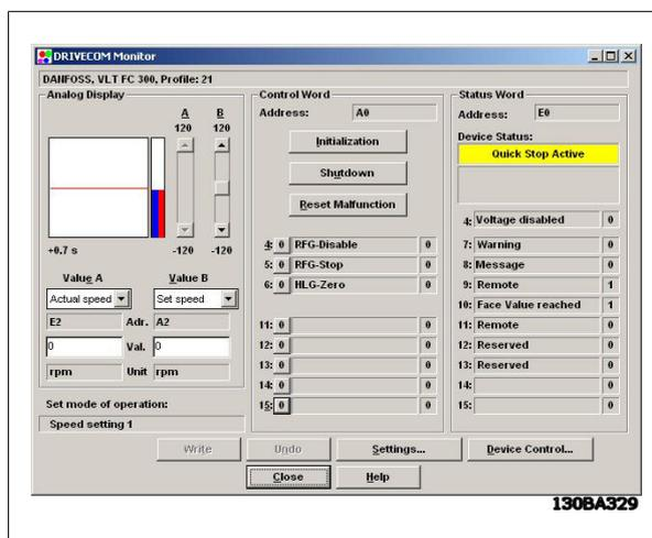
Click on Device Control to begin controlling the VLT frequency converter.
