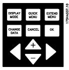
DISPLAY MODE [DISPLAY MODE] is used for selecting the indication mode of the display or when returning to the Display mode from either the Quick menu or the Extend menu mode. warning (WARNING) and alarm (ALARM), respectively. All frequency converter parameter Setups can be changed immediately via the control panel, unless this function has been programmed to be *Locked* [1] via parameter 016 *Lock for data change* or via a digital input, parameters 300-307 *Lock for data change*.
