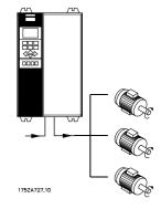
VLT 8000 AQUA is able to control several motors connected in parallel. If the motors are to have different rpm values, the motors must have different rated rpm values. Motor rpm is changed simultaneously, which means that the ratio between the rated rpm values is maintained across the range.
