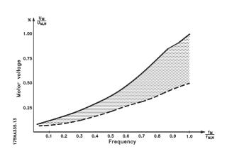
If the AEO function has been selected in parameter 101, *Torque characteristics*, this function will be constantly active. If there is a major deviation from the optimum U/f ratio, the frequency converter will quickly adjust itself.
