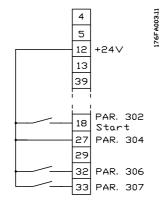
Selection of Setup using terminals 32 and 33.
