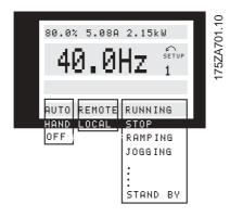
The left part of the status line indicates the control ele-ment of the frequency converter that is active. AUTO means that control is via the control terminals, while HAND indicates that control is via the local keys on the control unit.
