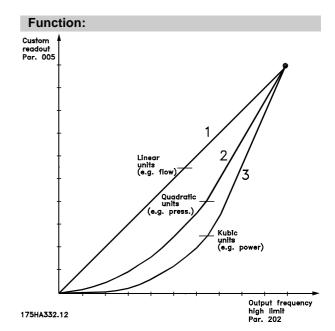
Select a unit to be shown in the display in connection with parameter 005 *Max. value of user-defined readout*. If units such as flow or speed units are selected, the ratio between readout and output frequency will be a linear one.
