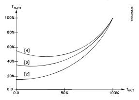
For constant torque loads such as conveyor belts, presses, mixers, screws and so forth, select *Constant*
