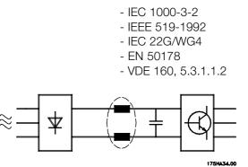
The voltage distortion on the mains supply depends on the size of the harmonic currents multiplied by the mains impedance for the frequency in question. The total voltage distortion THD is calculated on the basis of the individual voltage harmonics using the following formula:
