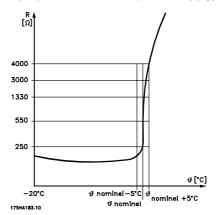
A motor thermistor connected to terminals 53/54 must be double isolated to obtain PELV.
