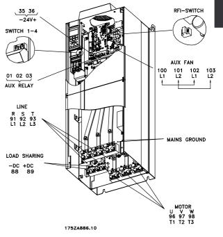
IP 00/Chassis VLT 8152-8202, 380-480 V VLT 8052-8202, 525-690 V Note: The RFI switch has no function in the 525-690 V drives. Installation
