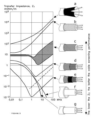
Transfer impedance ( $Z_T$ ) is rarely stated by cable manufacturers, but it is often possible to estimate transfer impedance ( $Z_T$ ) by assessing the physical design of the cable. Transfer impedance  $(Z_T)$  can be assessed on the basis of the following factors:
