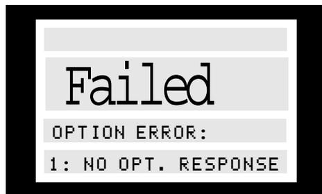
Try to reinitialize drive by removing power until display does blank. Reapply power. If drive functions are not restored, order the Danfoss EEBLANK Kit (P/N 175L4167) to restore the EEPROM functionality.
