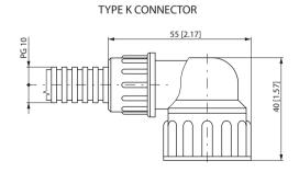
Standard connector to Kostal patern, for use with DC input. Type K Order no. 088010350
