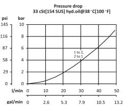
**Specifications** Rated pressure 207 bar [3000 psi] Rated flow at 7 bar 48 l/min [100 psi] [12.7 US gal/min] Leakage 6 drops/min @ Rated pressure Weight 0.12 kg [0.27 lb] Cavity SDC08-2
