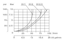
Values for adjustment H are guideline only, being conditioned by a variety of factors (oil temperature and viscosity, volume and flexibility of circuits).
