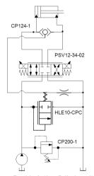
Double Acting Cylinder with Proportional Speed Control, Unloading Valve and Circuit Relief
