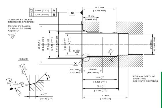
▼Caution SDC12-2 and CP12-2 (new name SDC12-2CP) cavities are not interchangeable. Differences in sealing area depth may lead to leakage if the wrong valve is used with this cavity. Use only the specified cavity for each valve.
