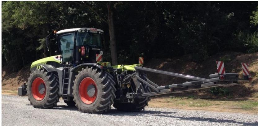
Figure 2: CLAAS Xerion 5000 with test plough rear and front weight.
