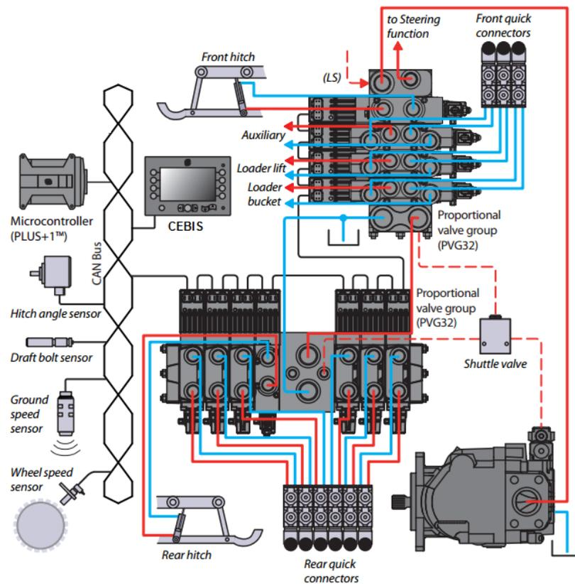
Figure 3: Hitch control system implemented on CLAAS Xerion 5000. Further details can be found in [15].
