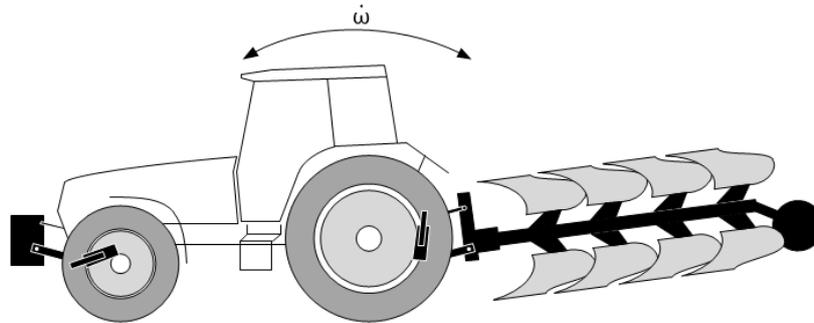
Figure 1: Pitching movement of an agricultural tractor with front weight and plough.
