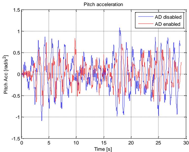
Figure 5: Comparison of pitch accelerations for plough implement.
