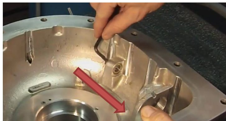
Figure 4. Worm Gear Removal
