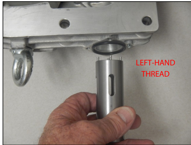
Figure 2. Locking Collar Tool Usage
