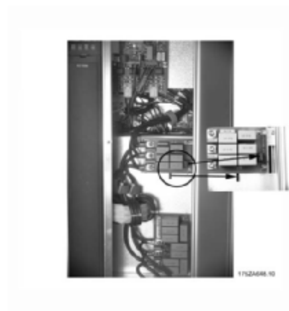
Position of RFI switches
