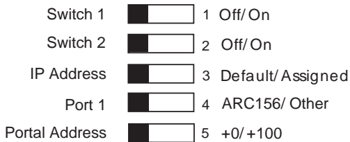
Figure 8. BACLink DIP Switches
