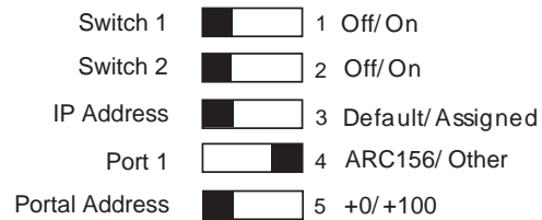
Figure 16. BACLink DIP Switches
