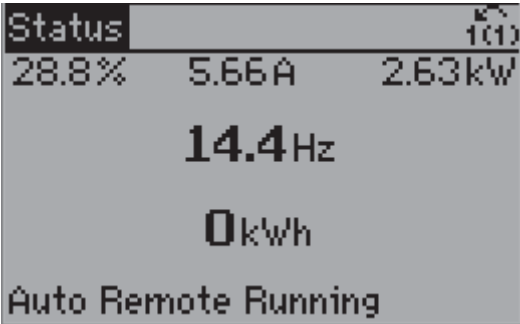
Illustration 6. 2: Step 1: Turn on the frequency converter (yellow LED lights)
