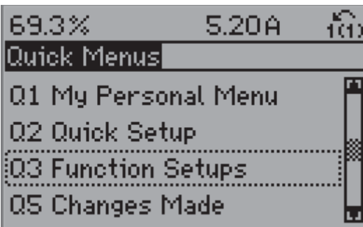
Illustration 6. 4: Step 3: Use the up/down navigation keys to scroll down to Function set-ups. Press [OK].
