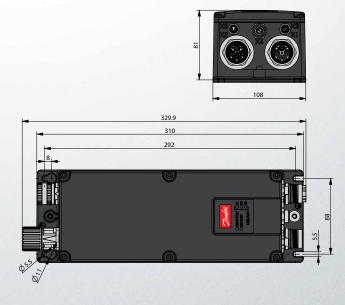
A = decoupling plates All measurements are in mm
