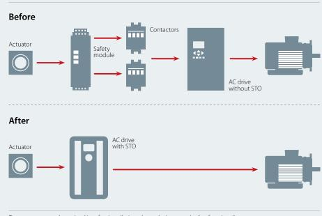
Two contactors can be omitted in safety installations due to the integrated safety functionality.
