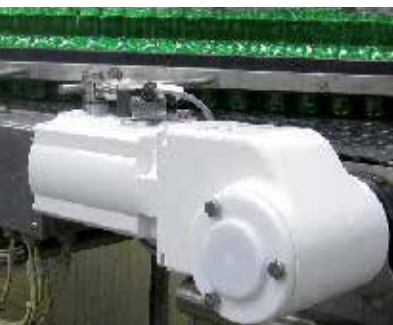
A cover is also provided for shaft ends used in gears for hygiene-critical areas.
