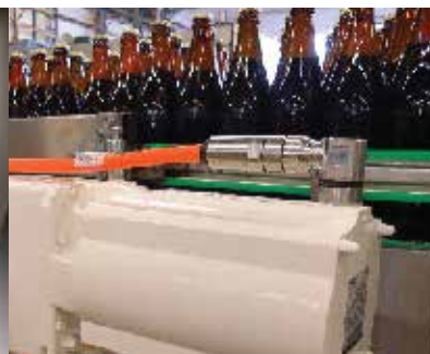
CleanConnect™ stainless steel connectors provide simple, safe connections even during replacement work.
