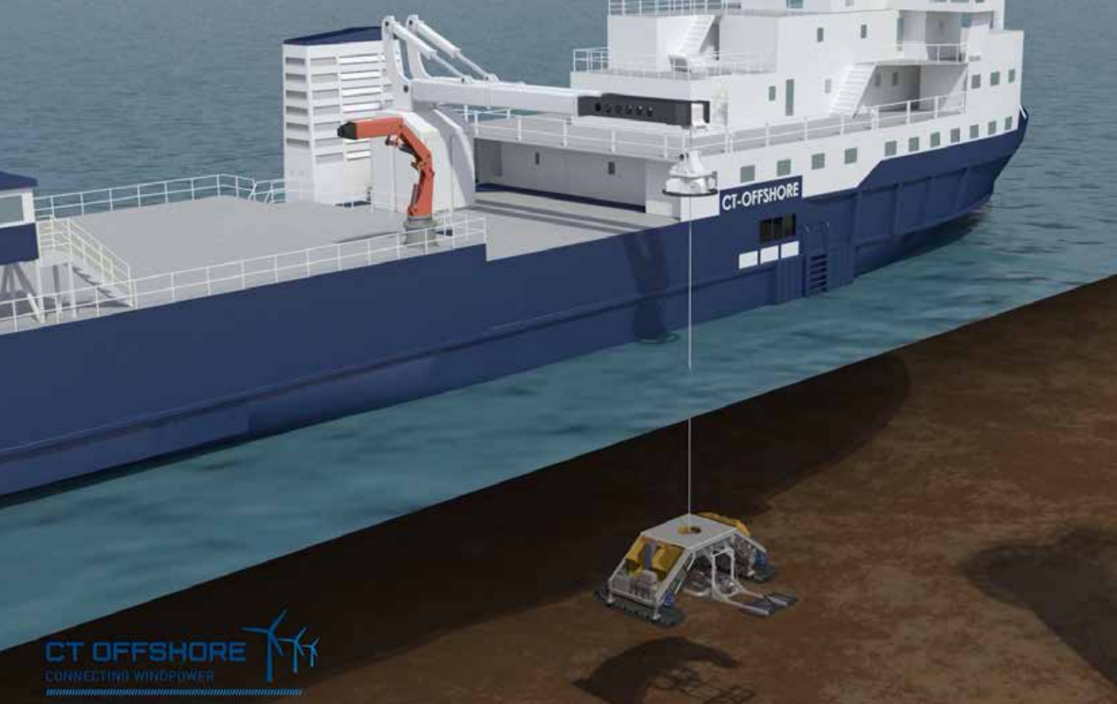
How the ROV is lowered to the sea floor
