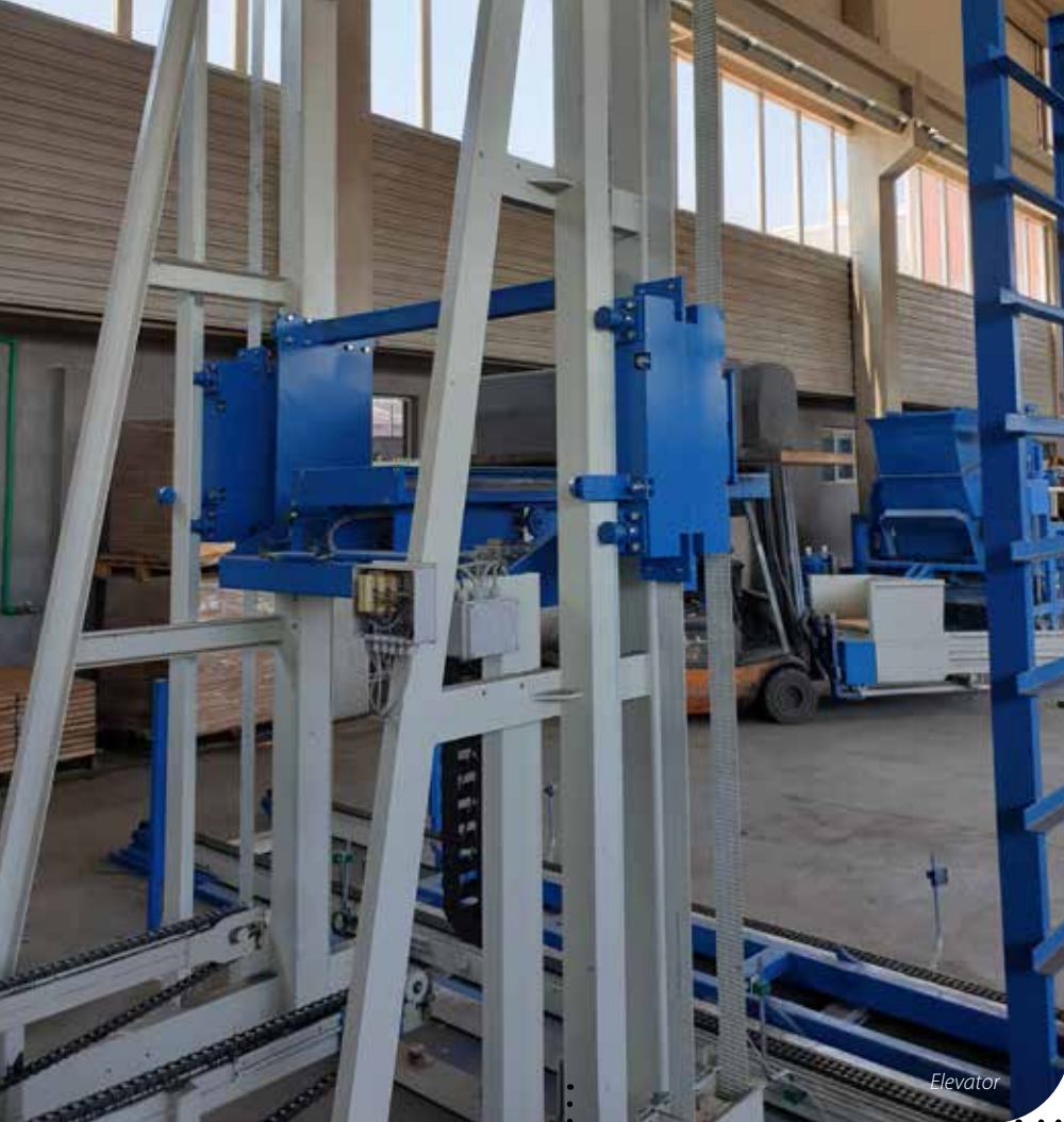
Elevator homing sensor to determine the zero point of the machine position
