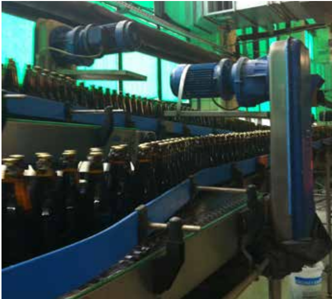
Before: Helical gearbox with chain and asynchronous motor
