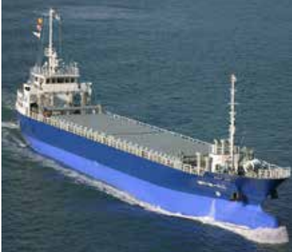
Mukaishima Dock's electric propulsion bulk carrier, with 499 gross tonnage and 1,800 deadweight tonnage, was built in Qingdao Shipyard located on Jimo Island in Shandong Province, China. Construction of the vessel began in March 2010, the ship was launched in September and sea trials took place in November 2010. This environmental-friendly vessel received a special subsidy from the Japanese government.
