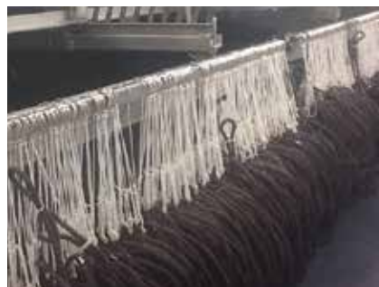
Longline fishing is a commercial fishing technique that uses a long line, called the main line, with baited hooks attached at intervals. The Northern Leader is capable of fishing 76,800 hooks using a Mustad Auto line Super Baiter designed by Mustad Longline AS in Norway. The length of line may stretch to 45 miles (72 km)!
