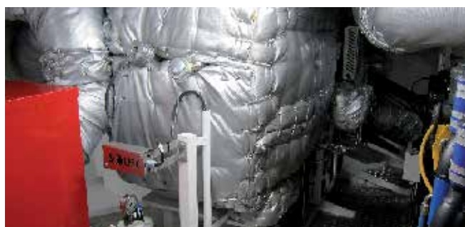
There are two 133 kW JohnDeere/Stamford generators in each engine room, four in total. The 2 engine rooms are located one at each end of the ship. The Solfic SCR exhaust gas filter removes toxic gases and particles.
