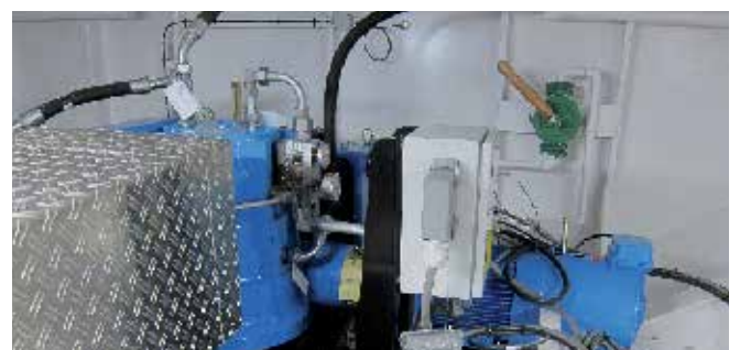
The ZF azimuth thruster (blue) is powered by an Oswald high-efficiency PM motor (green). Azimuth thrusters are often used in small ferries due to the good manoeuvrability they provide.
