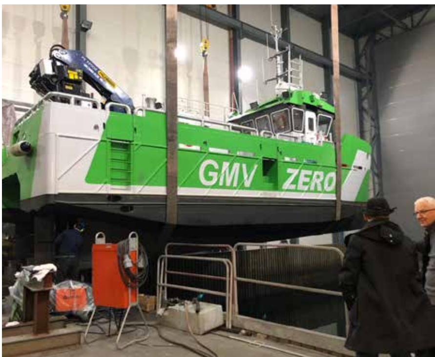
Astrid Helene is a 14-meter-long and 8-meter-wide aluminum catamaran workboat. Photo from the construction phase at Grovfjord Mekaniske Verksted.
