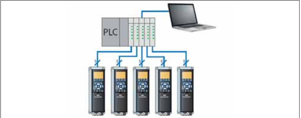
Fig. 8.7 Traditional wiring. No fieldbus
