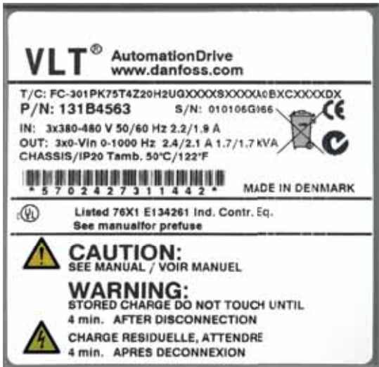
Fig 9.2 Identification data of a Danfoss frequency converter
