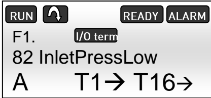
Figure 7.1-4, Low pressure alarm on the NXP panel
