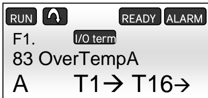
Figure 7.1-2, High temperature alarm on the NXP panel
