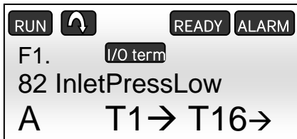
Figure 7.1-4, Low pressure alarm on the NXP panel
